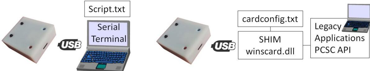
After software downloading LeMonolith is working in USB mode. Thanks to USB serial interface (115200 bauds, no parity, one bit stop) a *command shell* gives access to the secure element. It provides three main commands
