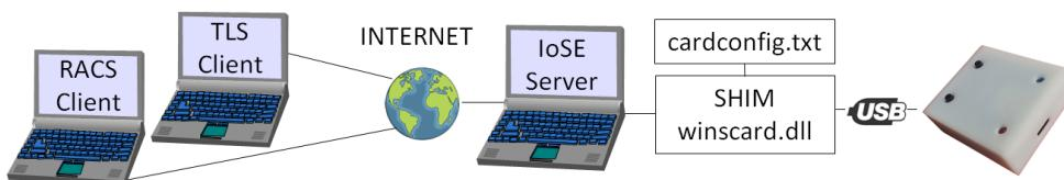
Internet of Secure Element (IoSE) server manages two TCP daemons: one for *Remote APDU Call Secure* (RACS) server (port 7777), and another for TLS1.3 front server port (8888). For windows the *winscard.dll* SHIM makes a bridge between PC/SC and USB serial. Within the IoSE server the secure element identifier (SEID) is 999, and the secure element name server (SEN) is *COMX001*.
